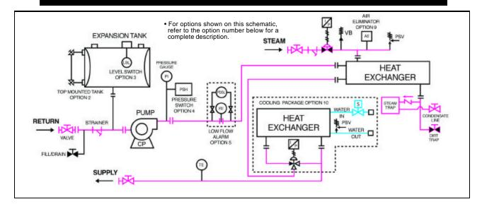
EM systems are custom designed and built to order. Designs are based on BTU/HR heat load, operating temperature, flow rate required, and available steam supply. The above diagram is typical and contains most of the commonly used components. The centrifugal pump is equipped with a mechanical seal and TEFC motor. Mechanical components include strainers, steam trap, relief valve, check valve, dirt
