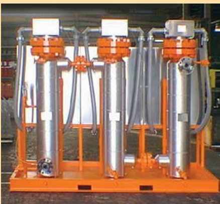
480 kW boiler water pre-heater
