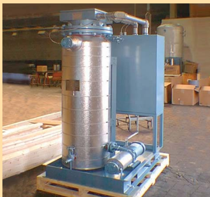
200 kW fuel oil pre-heater
