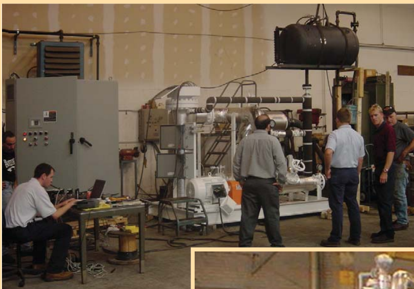
The above photo shows a 550°F hot oil system during the final operating test.
