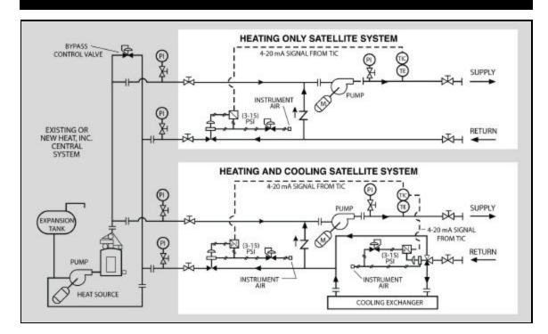
SS systems are custom designed and built to order. Designs are based on BTU/HR heat load, operating temperature, flow rate required and available hot oil supply. The above diagram is typical and contains most of the commonly used components. The centrifugal pump is equipped with a mechanical seal and TEFC motor. Other mechanical components include
